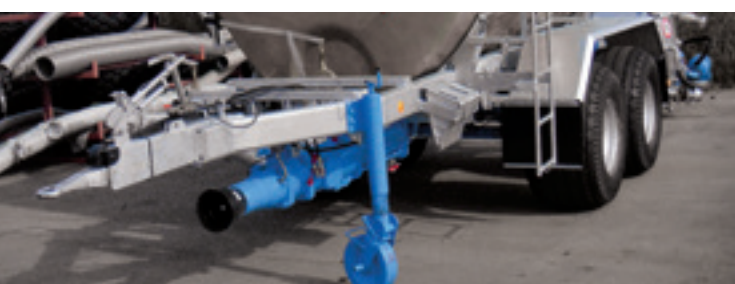
PTO pump on liquid manure tank / pump tank wagon
