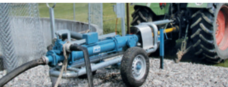
Umbilical system from a liquid manure tank with a pump from the WANGEN GL-series
