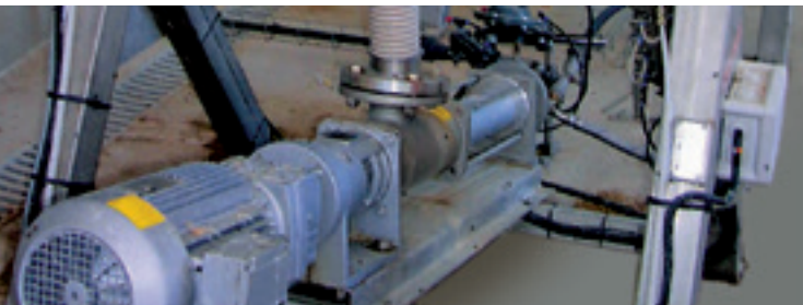
WANGEN KL30-S used with a liquid feeding system
